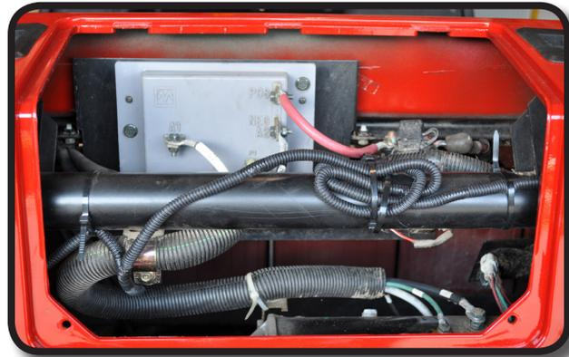
**IMPORTANT:** How you connect the wiring harness to your cart's battery pack will depend entirely on your cart's battery pack configuration. This light kit is intended for 12 Volt applications. Take care not to supply too much voltage to the unit as this will cause a failure that is not covered by manufacturer's warranty.
