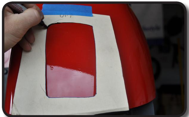
Drill a pilot hole and cut, again staying to the INSIDE or on the mark.
