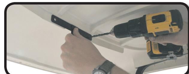
For Yamaha® Drive®, drill holes into canopy as shown.
