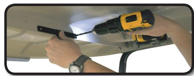
For Yamaha® G-SERIES®, drill holes into canopy as shown.
