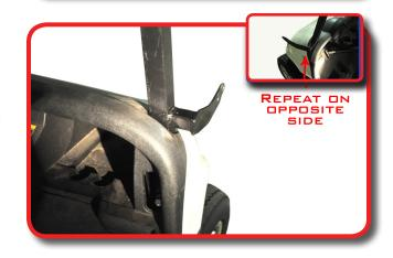
Attach Clays Basket using supplied hardware and tighten as shown.
