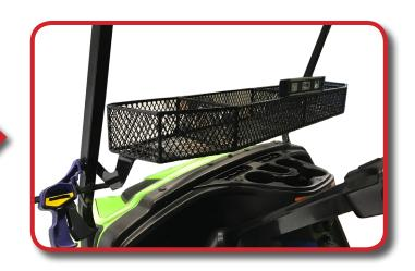
Drill hole through strut with 5/16" Drill Bit and secure mount basket with supplied 8mmx45mm bolts.
