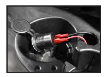
Insert USB into mounting hole and secure with the ring nut.
