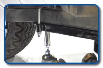
Using a 17mm socket, tighten U-Bolt hardware on front and center locations. Be sure hardware is tightened evenly.
