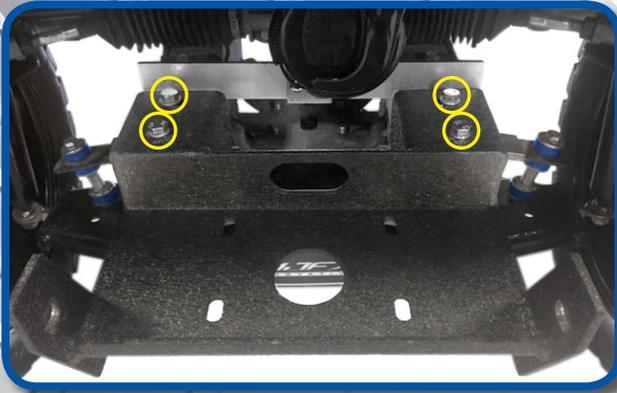
Place the Armor Bumper mounting bracket in place of the factory bumper. Attach using supplied 8mm hardware and two bolts retained from step 1. Tighten.
