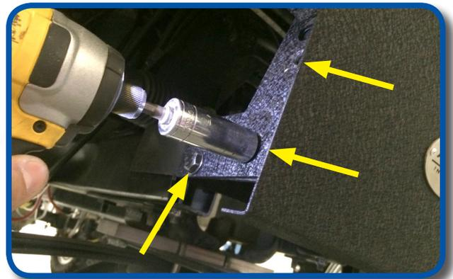
Before tightening the bumper, you can adjust the bumper to your specifications by using the slotted holes in the bumper and bracket. Once bumper is adjusted to your preferred location you may tighten all hardware.
