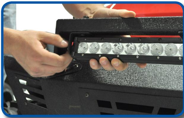
Make adjustments to tabs for the light bar to fit inside of and tighten brackets.
