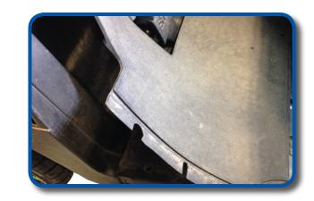
Using a small screwdriver pry the charge cover receptacle from vehicle and retain.
