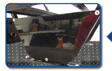
On the outside of seat frames secure the bottom of the seat panels using the screws in the seat frame.
