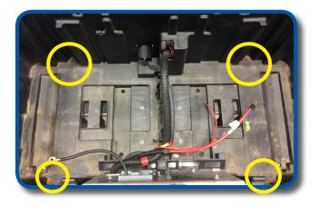
Remove four screws that secure the battery box to the frame and retain.
