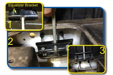
Remove turnbuckle and equalizer bracket by moving the buckle and bracket to the upright position. This will allow cable heads to slip out the top of the equalizer bracket. Retain buckle, Equalizer Bracket both washers. Discard threaded rod. Disconnect any brake light cables and disconnect two MCOR connectors.
