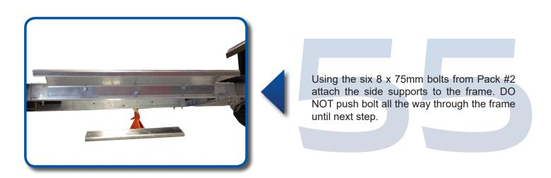
With side supports hanging, slide center floor support between frame rails and push bolts from previous step through frame into center support. DO NOT tighten until all 6 bolts are in place. NOTE: Make sure predrilled holes on top of center support are off set to the FRONT of the cart.
