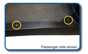
Locate the two front screws as well as the back screw/rivet in the floormat retainers. Remove retainers, save hardware and retainers.
