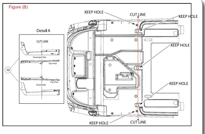
Measure, Mark, and Cut Front Underbody (Save the Holes indicated by Arrows)
