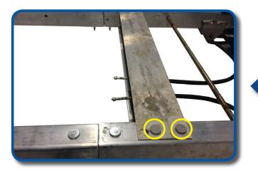
Before installing new carriage bolts into frames, reattach cross frame support using hardware retained from step 42.
