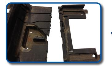
Remove the under body from cart and finish cutting along chalk line where the frame was.
