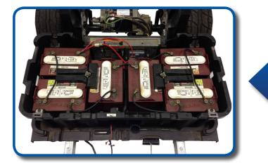
Reinstall battery pack and secure with battery blocks and hold downs.
