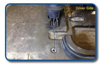
Using a reciprocating saw and a metal cutting blade between 8-10". Begin cutting along your chalk line from the outside of the under body to the outside of the first frame. DO NOT CUT FRAME. NOTE: Cut vertically and from the top side of the vehicle.
