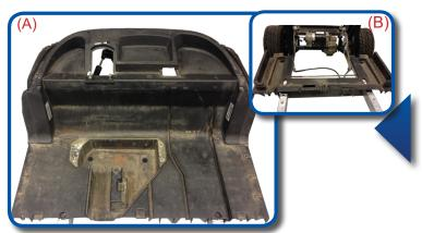
(A) Re-attach front under body using hardware from step 39
