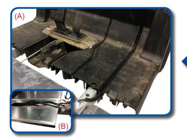
(A) Attach IP 12 Pin harness extension and run through underbody channel to front dash.(B) Make sure 12 pin connectors are joined together where center support and front underbody gaps.
