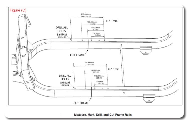
NOTE: Use Figure (C) as a guide. Using the rearward most mounting hole, measure forward and mark the center of the three new holes needed in Figure (C) Once holes are marked use a center punch at the center mark of the frame as a drill point.
