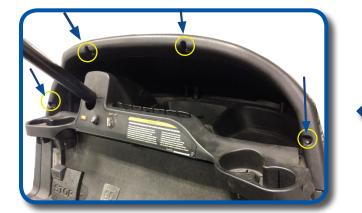
Remove brow cap by taking out the four screws as shown and retain. Remove cowl from front of cart and retain.
