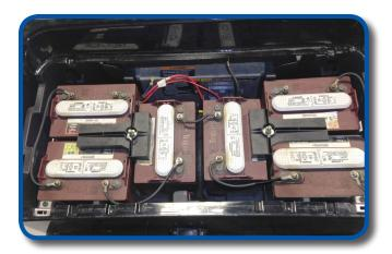
NOTE: We recommend taking a picture of battery layout and wiring pattern before disconnecting and removing batteries. Disconnect and remove the battery inter connecting wires and retain.
