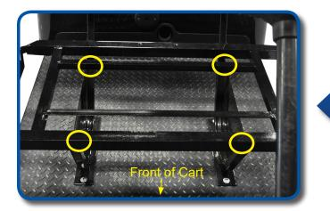
Attach seat support bracket to seat frames using four 8mm x 45mm bolts and hardware from Pack #4. Tighten hardware. Attach rear cup holder to seat support bracket using two 8mm x 25mm countersunk bolts and hardware from Pack #4.
