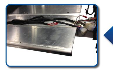
For carts 2008.5 and newer route bucket harness in same "V" channel as factory harness. Excess harness will need to be tied together in channel so 12 pin connector will equal factory 12 pin connector location from previous step.
