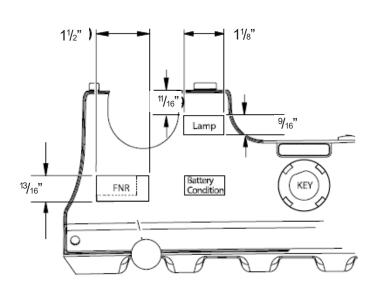
Make a  $1^{1}/8^{\circ}$  wide x  $9/16^{\circ}$  tall hole to the right of your steering column and attach the battery warning lamp as shown in Figure D.
