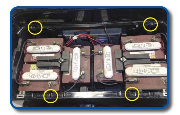
Detach the rear body by removing the four screws as shown. Retain all.
