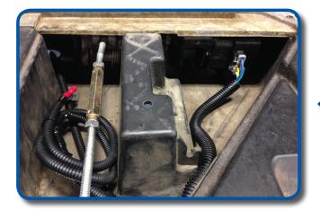
Feed brake pad plugs into pedal box and secure. You can now attach your harness plugs to the brake pad plugs if applicable. (A) Re-attach brake pedal cover.
