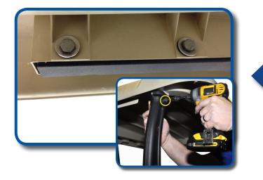
Detach canopy by removing the 6-bolts in struts. Retain Hardware.
