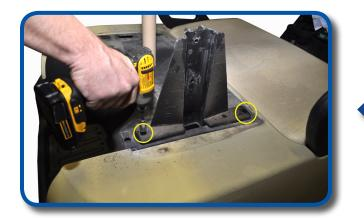
Remove hardware from basket retainer. Remove basket retainer. Retain hardware.
