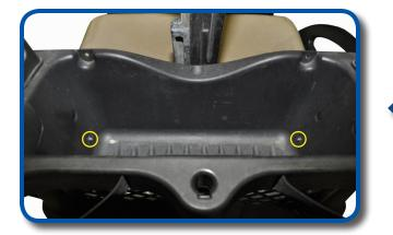
Remove lower rear strut hardware located on inside of basket. Remove factory struts. Retain hardware.
