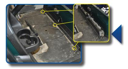
Remove the floor cover plate by taking out the three screws as shown. Retain all.
