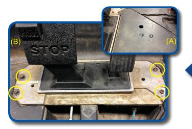
(A)Remove and retain brake pedal cover.(B)Remove four screws in pedal assembly. Retain all.
