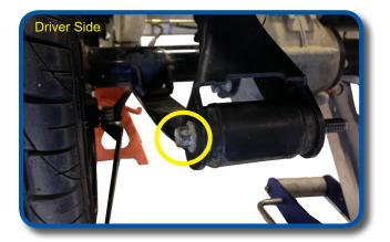
Carefully remove <u>rear</u> leaf spring bolt/nut and retain. NOTE: If floor jack is not in place the motor will likely roll and add difficulty when reattaching rear axle. Assemble jounce bumpers to jounce brackets. Now slide jounce under axle as shown.
