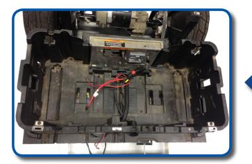
Reattach battery box to the frame using retained hardware from step 28
