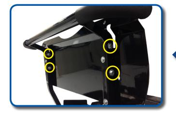
Attach rear grab bar using four 6mm x 40mm bolts and hardware from Pack #5 as shown. Once all four bolts are in place, tighten. Attach front seat back using retained hardware from step 3 and two 6mm x 20mm bolts and hardware from Pack #5 as shown.
