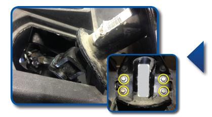
Remove the 4 bolts that attach the steering column to the frame. Retain Hardware.
