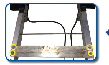
Remove 4 bolts from cross frame and retain all. Slide cross frame off of vehicle frame.
