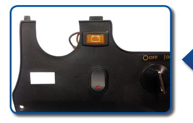
Enlarge the existing battery warning lamp hole for the F-N-R switch. New dimensions should be 1.5" wide x 13/16" tall. Refer to Figure D if needed.
