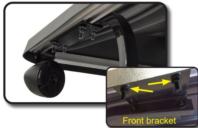
Connect the strut brackets to the top extrusion using 8mm carriage bolts, hand tighten hardware first. Once all bolts are in place then tighten.
