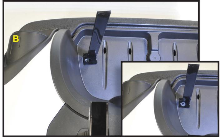
C) Attach bagwell bracket using retained hardware.
