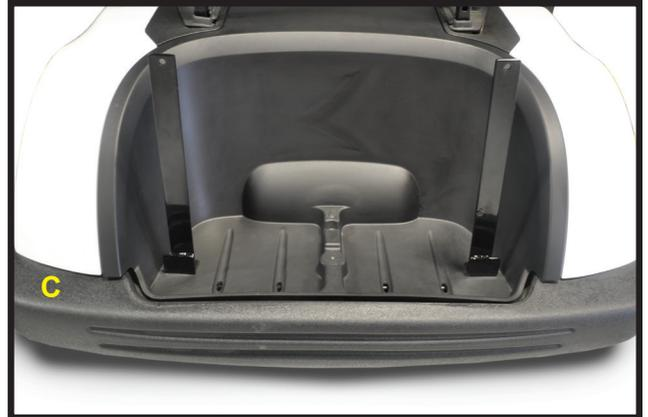
Attach cargo box bracket to main bracket using 10mm x 45mm hardware provided, hand tighten.
