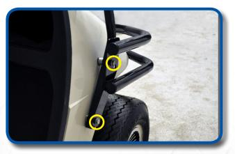
Using retained factory hardware, attach brush guard to front struts. Tighten bolts.
